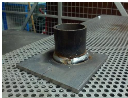
Fig. 88. - Welding Result in the circular joint
