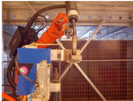
Fig. 95. - Stage 1. Wire cutting
