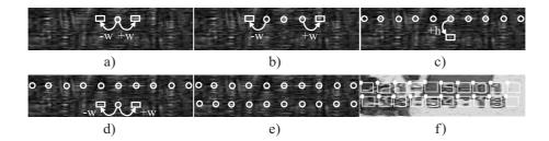
**Fig. 4.** Character location and segmentation algorithm. Starting from the overall maximum matching, a), the process moves left and right searching for local maxima, b) and c), until it reaches the extremes. Then, we move below and repeat the process, d) and e). The resulting segmentation is shown in f).
