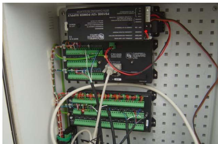
Figura 3.4: Datalogger CR1000 (Campbel Scientific)
