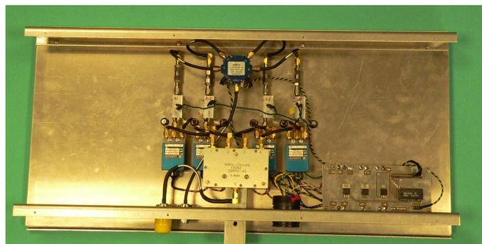
Fig. 4.69 – Array receptor, vista trasera
