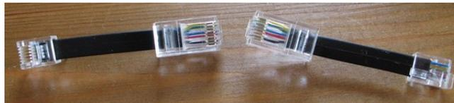
*Figura 3.6. Cables RJ12/RJ45.*
