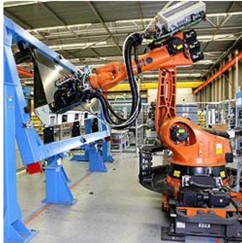
Fig. 2.1: A KUKA robot drills and installs fasteners in aircraft components [WEBKUKACOMP].
