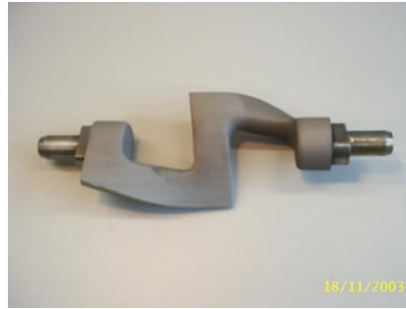
Fig. 1.11: Sigma-form blade for injection molding application.
