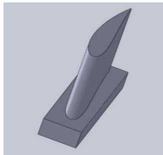
Fig. 6.15: Airfoil section NACA 5020 in CAD format.
