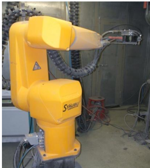
Fig. 1.5: Robot RX 130 (Co. Stäubli) for the coating in IFKB.
