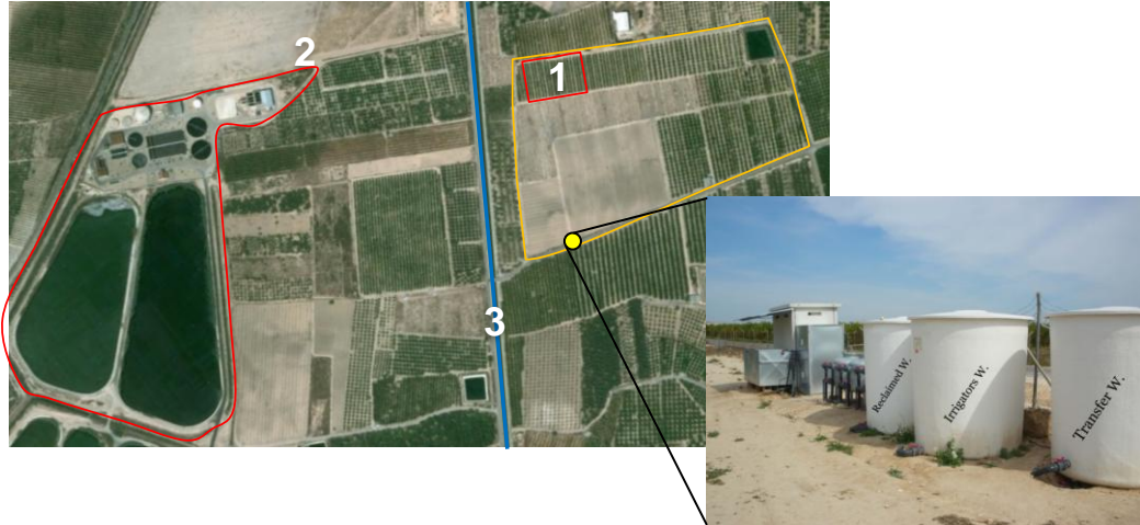
Picture 12. Irrigation control-head, equipped with 3 reservoirs, 3 sand filters and 3 disk filters. 1) Mandaine experimental plot, 2) Wastewater treatment plant of the “north of Molina de Segura”, and 3) Tajo-Segura water transfer canal.
