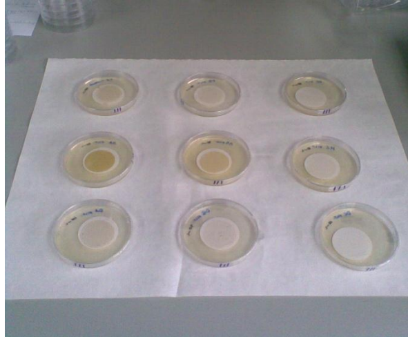
Picture 10: Fecal coliforms and E. coli isolated after incubation for 24 h at 44.5 and 37 °C, respectively.
