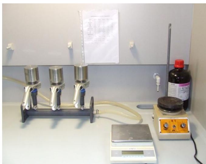
Picture 9: Microbial water analyses through a vacuum system filtering a sterile 0.45-µm-pore-size membrane filters.
