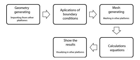
The first part of this calculus process consists of geometry generating, in what concerns us, the hull of the ship. It is usually imported from other platforms to CFD codes by means of different exchange files: iges, 3dm, dfx, aciis, parasolid... So, it will only be necessary to create a control volume for solving the studied problem. In our case, in the ship, the control volume should be a parallelogram formed by two parts: one for the water and another for the air.
