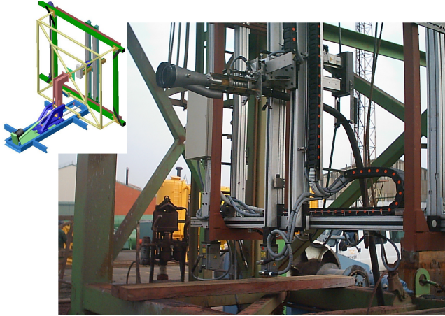
Figure 5. Cartesian robot developed in the context of the EU 5 th FP project EFTCoR for ship hull cleaning.
