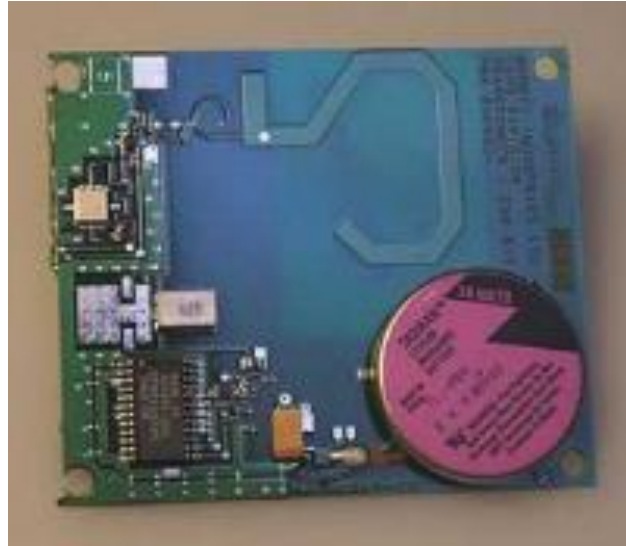
Figure 12: UHF RFID Semi Passive Tag
