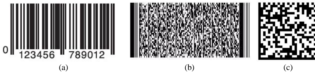
Figure 2: the different types of bar codes: (a) one-dimensional or linear, (b) stacked linear, (c) two-dimensional
