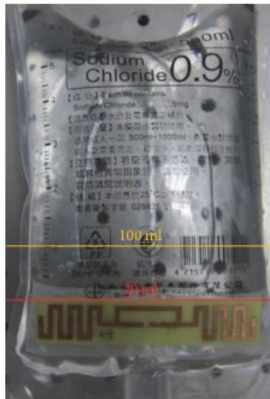
Figure 74: The proposed tag placed on full IV solution bag [21].
