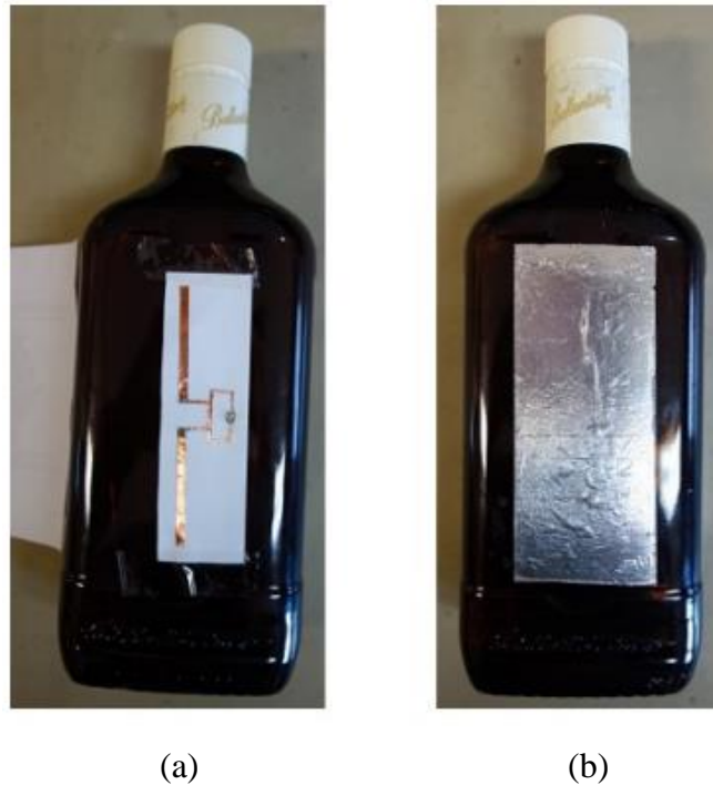
Figure 52: The proposed RFID tag antenna in the bottle. (a) RFID tag, (b) added reflector on back of bottle [5].
