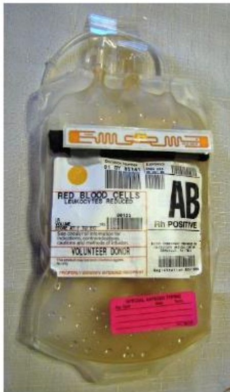
Figure 57: Commercial tag the “ALN-9640” placed on blood bag [15].
