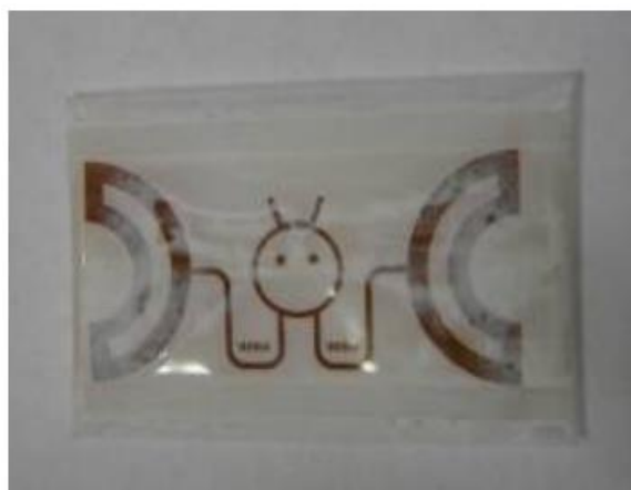
Figure 45: a commercial tag antenna with polyimide humidity sensing material
