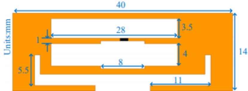
Figure 64: The proposed tag antenna [20]
