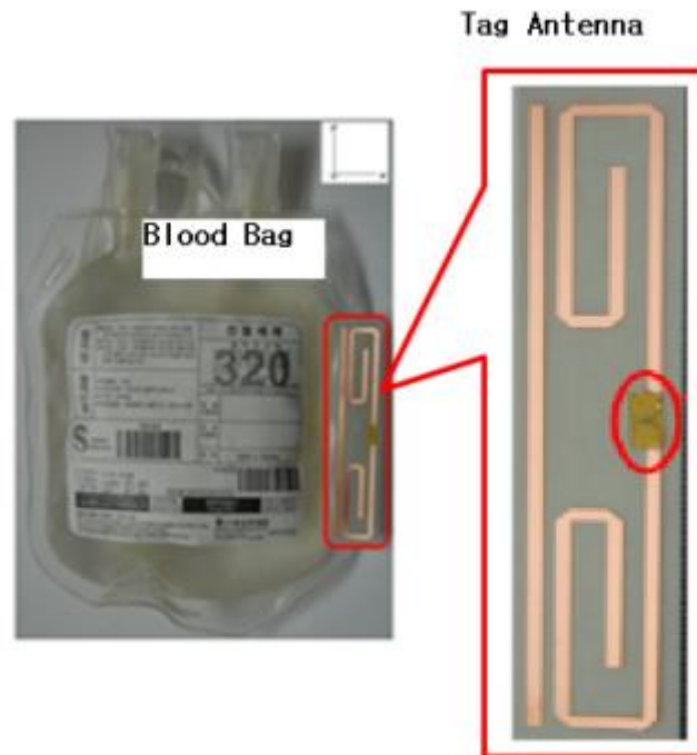
Figure 60: The geometry of a proposed tag attached on a blood bag [18].
