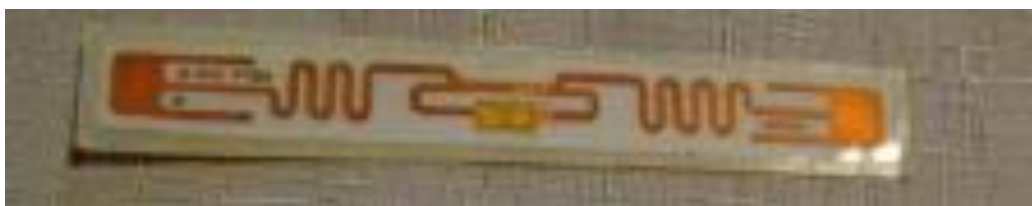
Figure 56: Commercial tag the “ALN-9640” from The Alien Technology [15].
