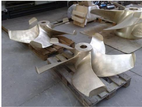
Figura 44: Hélices CLT.
