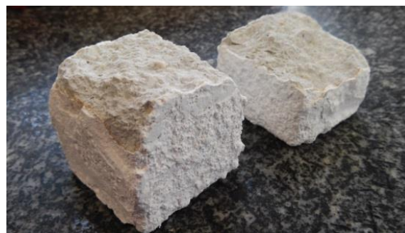
Figure 5. (a) X-ray diffraction spectra of control mortar and D mortar (with crystalline admixture) after 90 days of sulphuric acid attack; (b) Specimens exposed to the acid attack after compressive strength testing at t_{118(90)} , where the massive formation of gypsum in the surface of the specimen can be seen.
