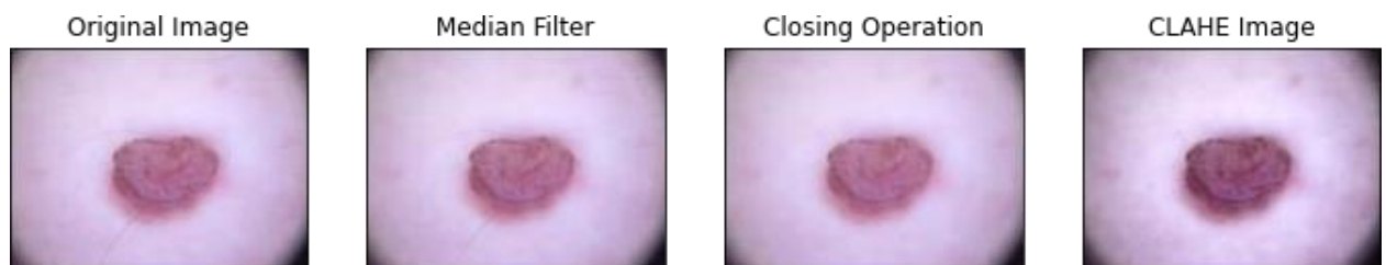
Fig. 40 Comparison between all the pre-processing steps of the benign lesion, since the original image (the one in the left), until the image after the application of the CLAHE method.
