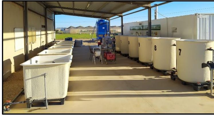
Figure 5.1. Citrus woodchips bioreactors in the pilot plant at the Agri-food Experimental Station Tomás Ferro (ESEA) of the School of Agricultural Engineering, Technical University of Cartagena (ETSIA - UPCT) to denitrification experiment with brines.
