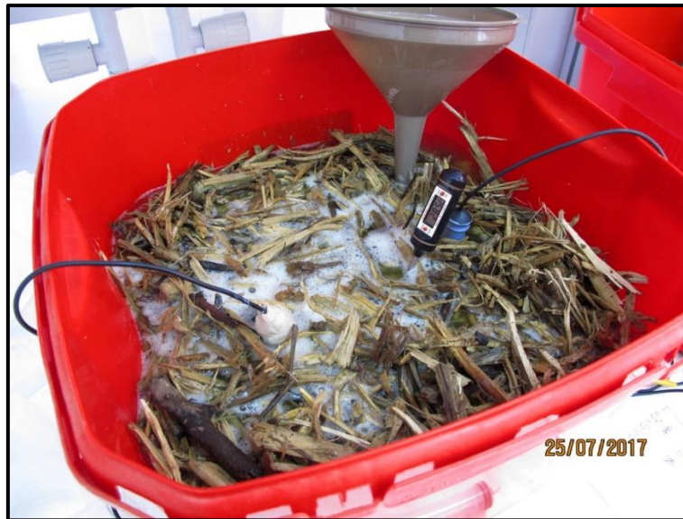
Figure 4.6. Detailed view of the thermometer and pH/Eh electrodes used in the batch bioreactors assays.
