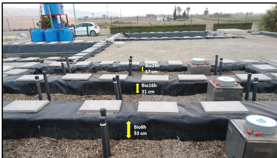
Figure 7.11. Detail of woodchips levels on day 566 of the experiment.
