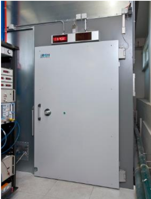
Dual-knife, 4 rows of Be-Cu fingers contact
