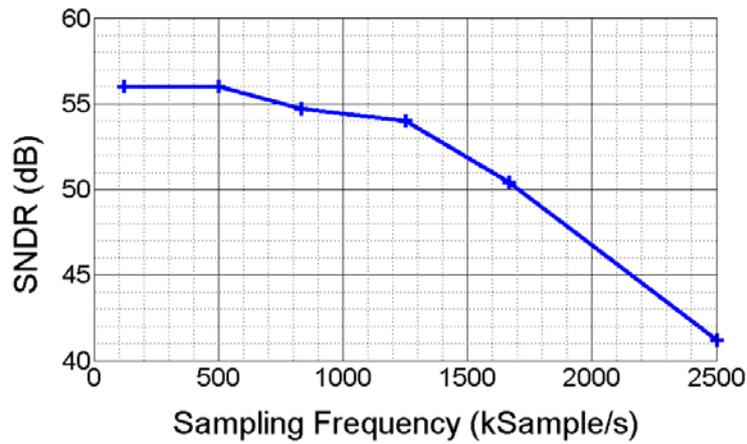
**Fig. 8** Dynamic performance of the ADC versus sampling frequency at f<sub>IN</sub> of 56Hz.
