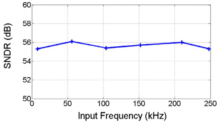
**Fig. 7** Dynamic performance of the ADC versus input frequency at f<sub>S</sub> of 500 kS/s.
