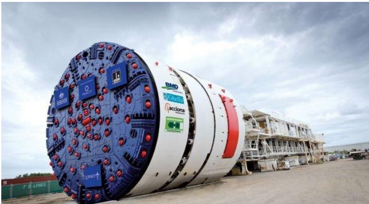
Figure 41. Cutting head TBM
