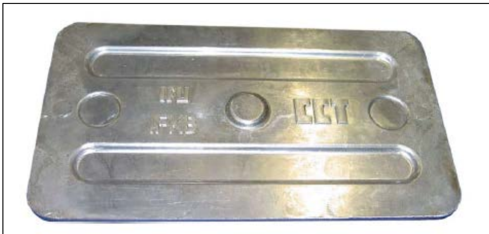
Figure 1.6 Thixo-forged, woven carbon fibre reinforced MMC with AlSi6 matrix, 214 x 124 mm [Gadow, 2010]
