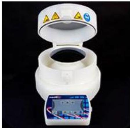
*Figura 33. Spin coater 150i/200i infinite.*
