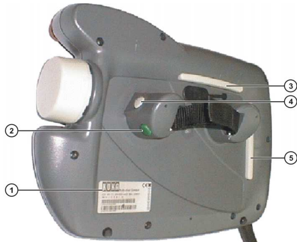
Picture 2.7. Rear of KCP.
