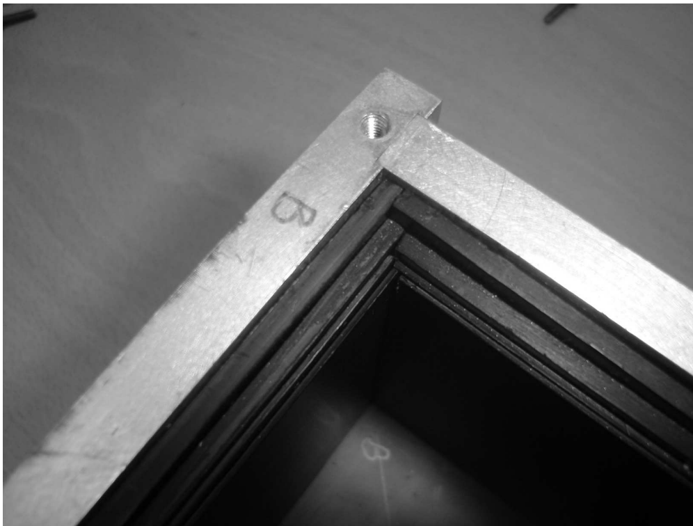
Four-layer conductive plastic structure inside a metallic cabinet 575x431mm (72 x 72 DPI)
