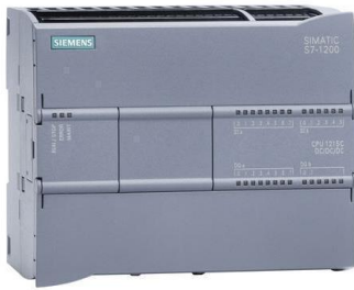
Figura 5. PLC SIMATIC S7-1200
