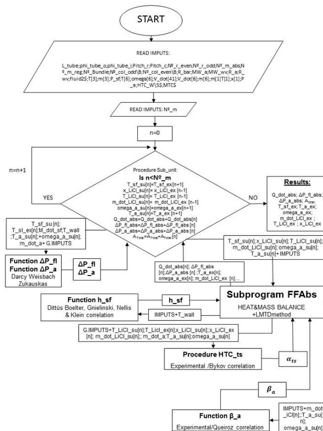
Figure 3. Architecture of the LDC model.
