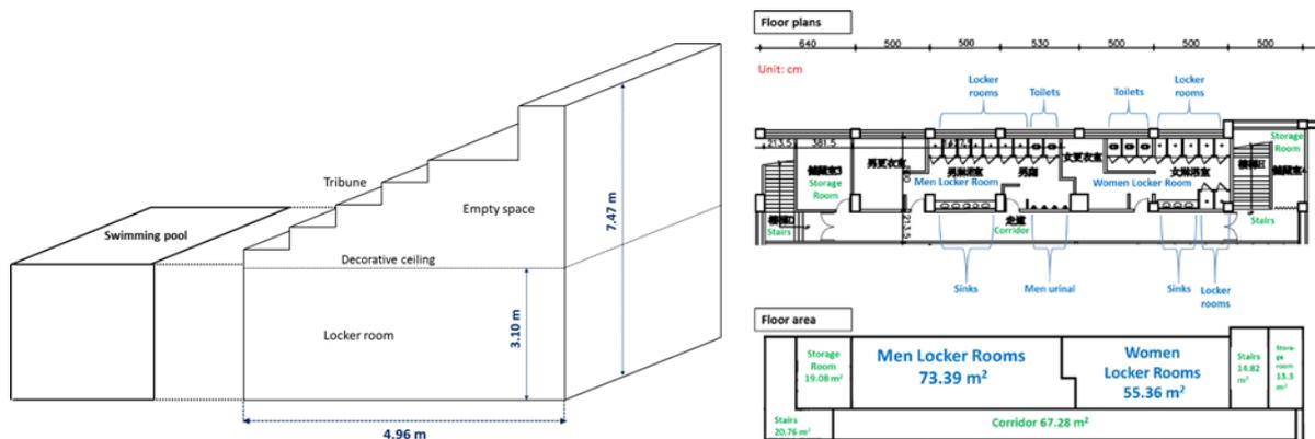
Figure 2. Location and distribution of the locker rooms of Taiwan Building Technology Center in Taipei
