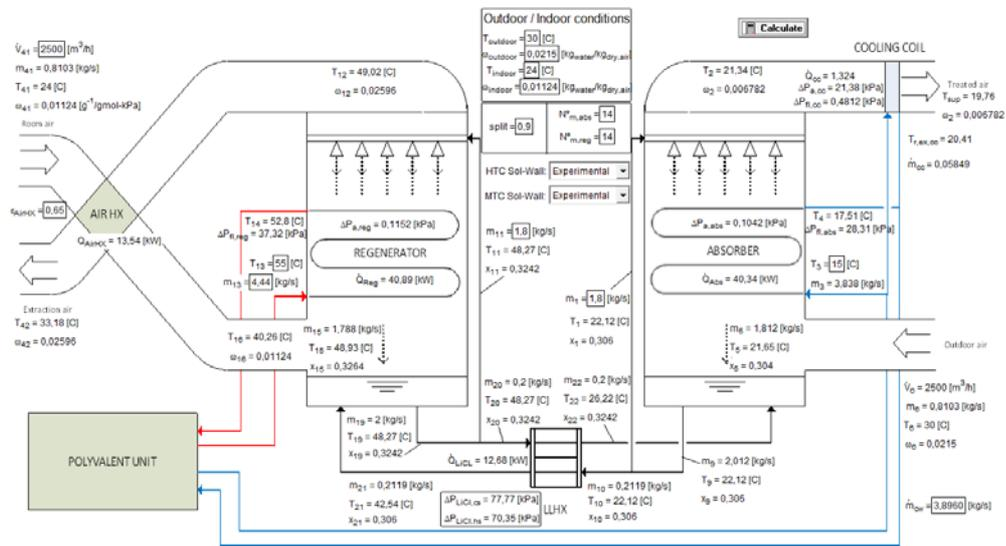
Figure 5: Results from simulation of the HLDS.
