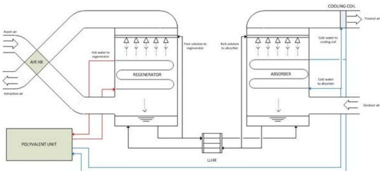
Figure 1. Hybrid liquid desiccant cooling system.
