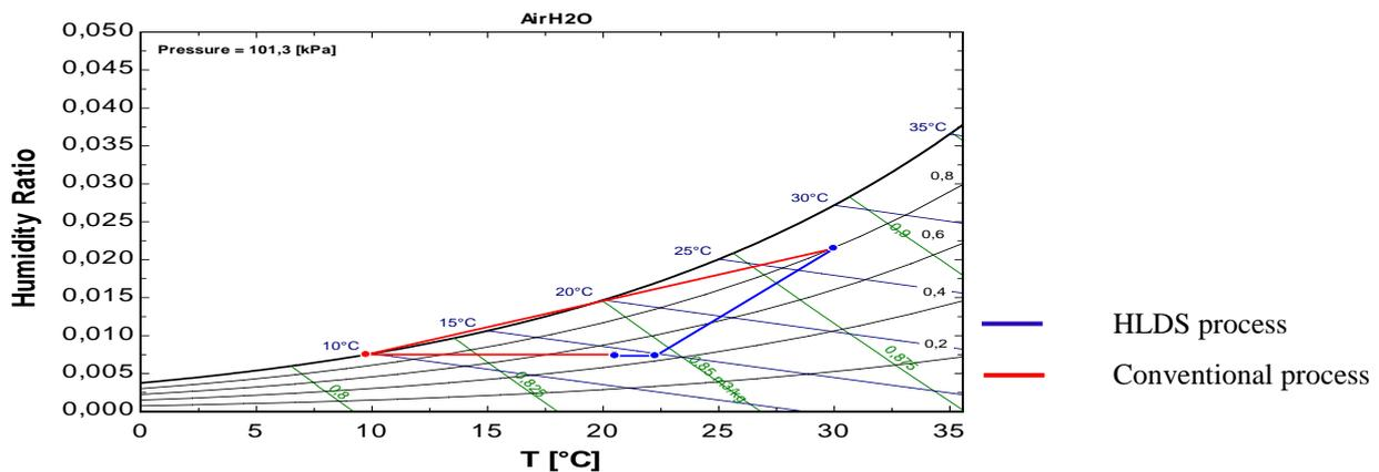
Figure 6: Air treatment processes in the HLDS and in a conventional cooling system.
