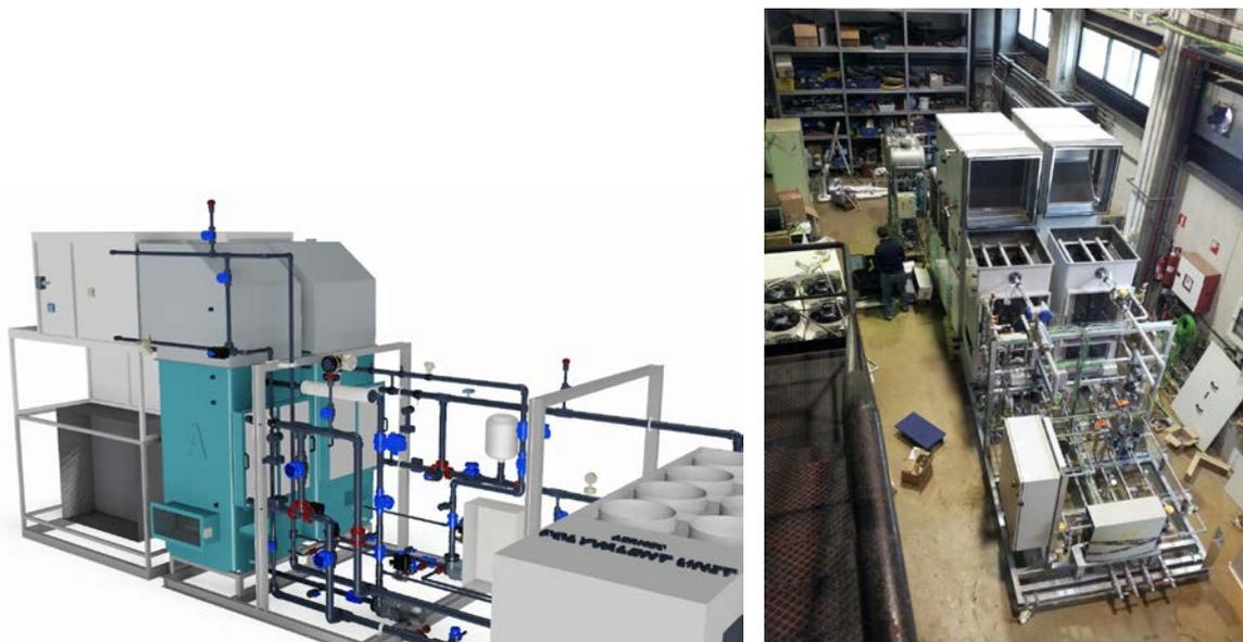
Figure 7:3D CAD design and prototype of the HLDS in the laboratory
