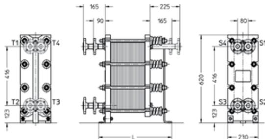
Figure 4: Liquid-liquid heat exchanger. SGL
