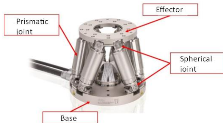
Figure 1. Parallel robot and its fundamental parts
