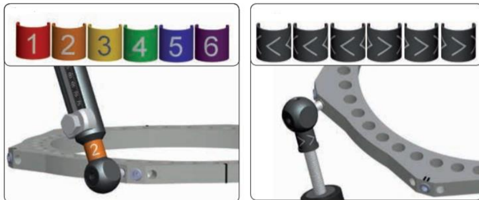
Figure 8. Built-in clip types
