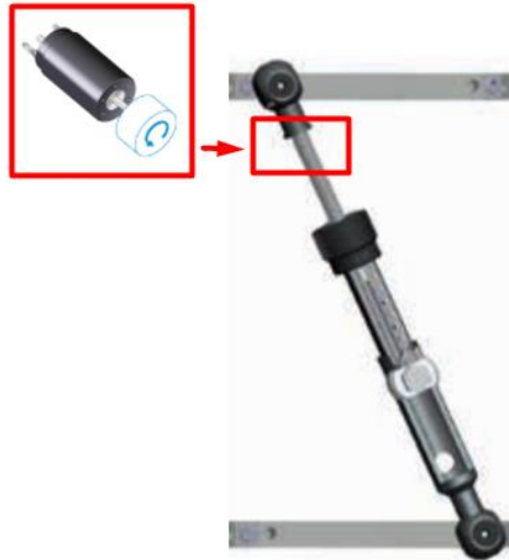
Figure 41. Location of the motor in the actuator
