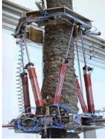
Figure 12. Climbing robot with pneumatic actuators for maintenance and fumigation of palm trees
