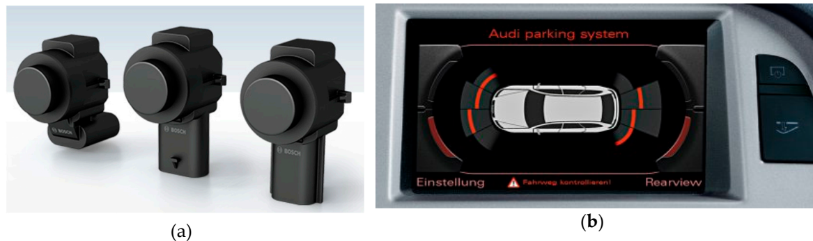
Figure 3. (a) Ultrasonic car sensors from Bosch; (b) an assistance parking system from Audi.
