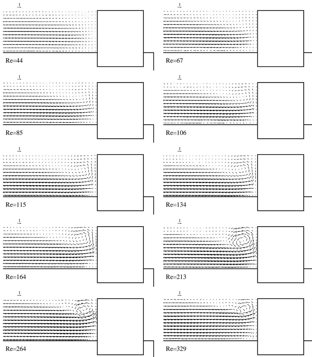
*Fig.5 PIV velocity field. Static device. Flow detail upstream the semi-circular element.*
