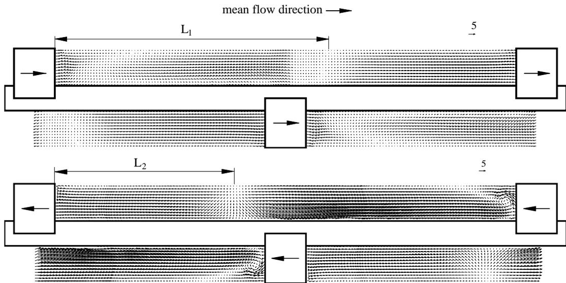
Fig. 6 PIV velocity field. Dynamic device at Reynolds numbers 44. Scraping velocity is three times the mean flow velocity ( $r=3$ ).
