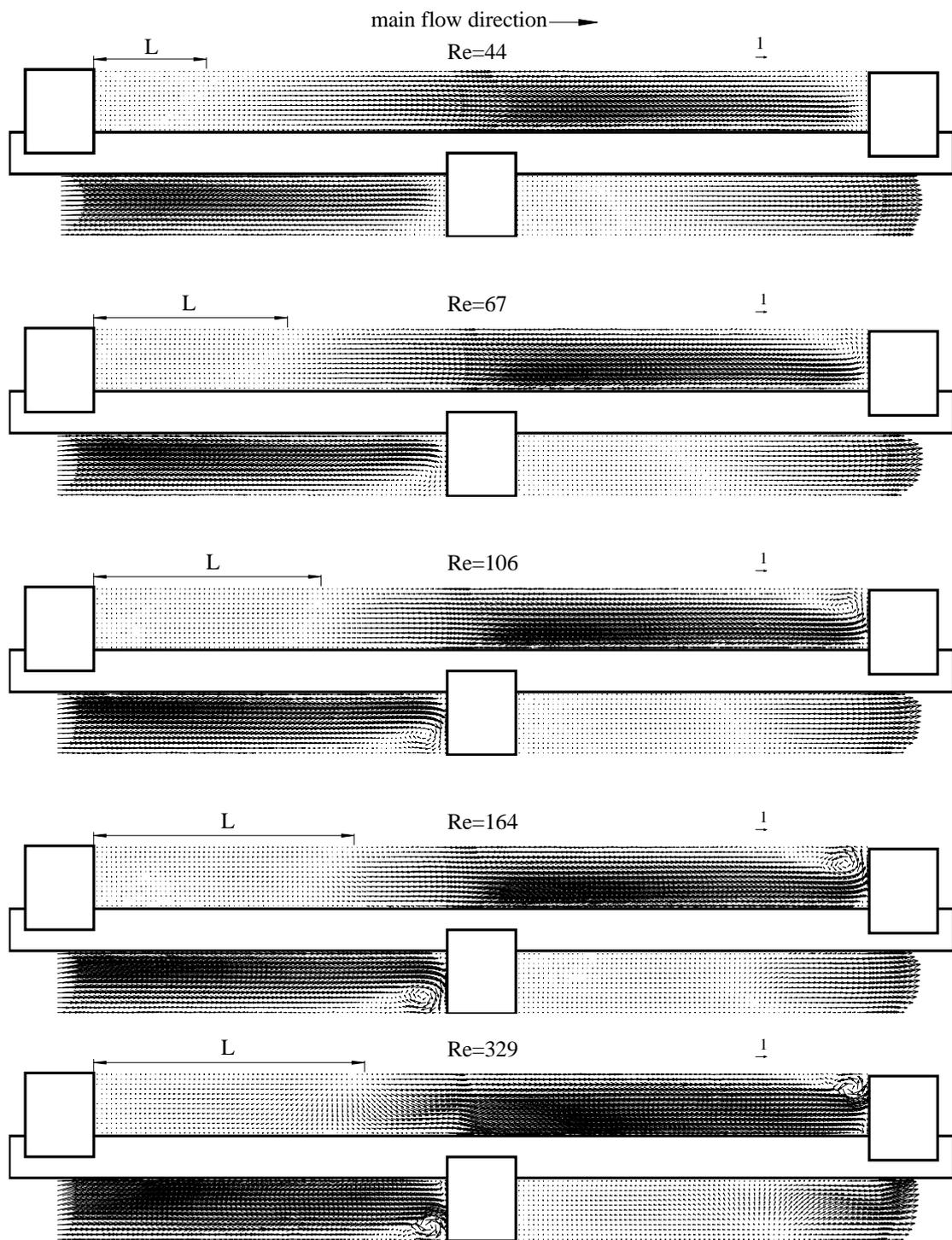
*Fig.4 PIV velocity field. Static device at Reynolds numbers from 44 to 329.*
