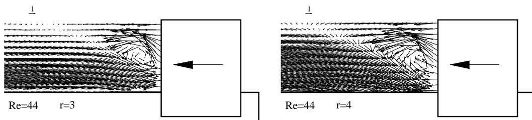
Fig. 8 PIV velocity field. Dynamic device at Reynolds numbers 44. Flow detail upstream the semi-circular element
