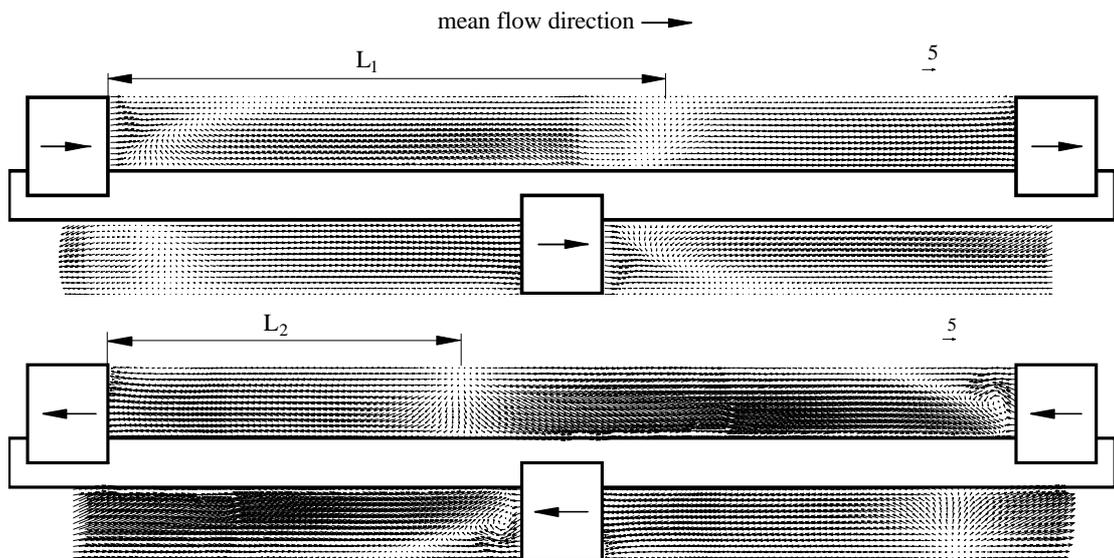
Fig. 7 PIV velocity field. Dynamic device at Reynolds numbers 44. Scraping velocity is four times the mean flow velocity ( $r=4$ ).
