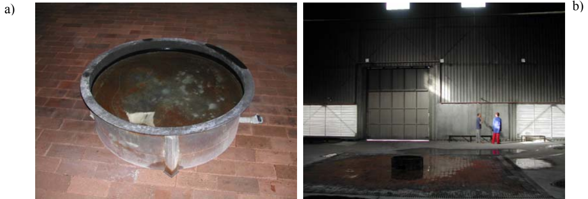
Figure 3. Pool-fire with D = 0.92 m and H = 0.2 m, in a), and test topology, in b).
