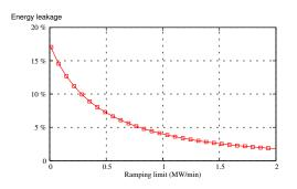
Figure 7: Energy leakage produce by the use of a positive ramp limitation.
