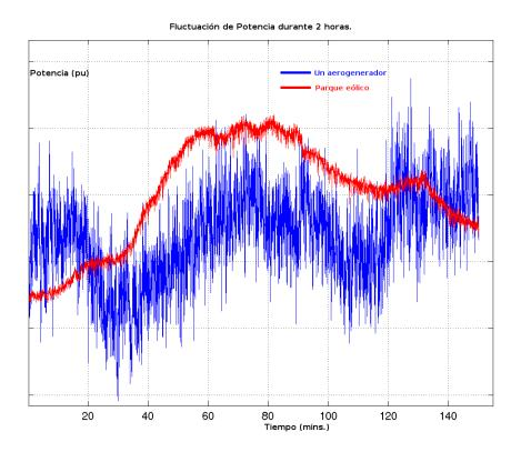
Figure 1: Example of power fluctuation when the wind farm is working under the nominal power.
