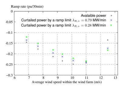
Figure 10: Comparison of the 99%-percentile of the ramp rates for the available power and the curtailed power with a positive ramp limitation characterised by  $\lambda_{R,+} = 0.79 MW/min$  and by  $\lambda_{R,+} = 0.28 MW/min$ .
