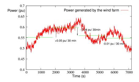
Figure 3: Example of ramping rates of the fluctuations in the power produced by a wind farm.
