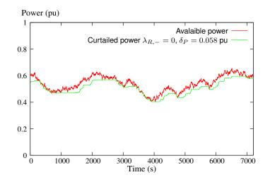
Figure 6: Example of the application of a delta constraint linked with all negative ramp limitation ( $\lambda_{R,-} = 0$ ,  $\delta_P = 0.058 \, pu$ ) to 2 hours of simulated available power.
