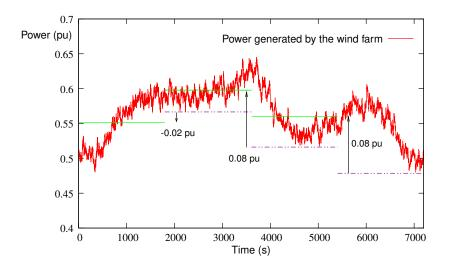
Figure 4: Example of reserves requirement due to the fluctuations in the power produced by a wind farm.
