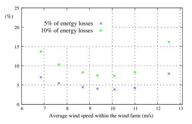
Figure 8: Comparison of the reduction of the reserve requirements (1%-percentile) for the curtailed power with delta+negative ramp limitation characterised by  $\lambda_{R,-} = 0$ ,  $\delta_P = 0.031 \, pu$ ; and by  $\lambda_{R,-} = 0$ ,  $\delta_P = 0.058 \, pu$  with regard to the available power.
