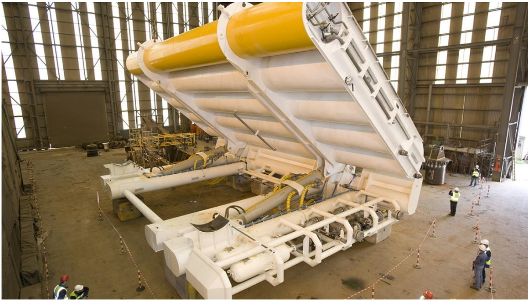
Figura 17. Sistema undimotriz Oyster. Tomada de (University of the Basque Country, 2018)
