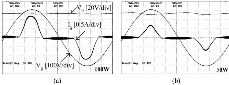
Fig. 17. Input current and output voltage without control loop for the line voltage ( $230 V_{rms}$ ) and  $K = 0$ . (a) Full load. (b) Half load.
