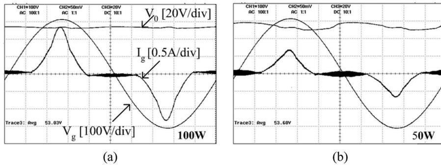
Fig. 18. Input current and output voltage without control loop for the line voltage ( $230 V_{rms}$ ) and  $K = 0.5$ . (a) Full load. (b) Half load.
