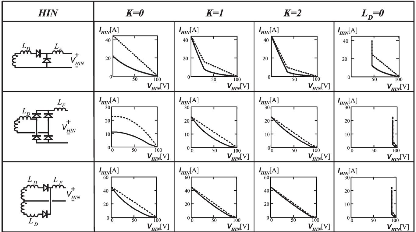
Fig. 14. (Dotted line)  $VCC_{peak}$  and (solid line)  $VCC_{AVG}$  for the HINs that are shown in the leftmost column.
