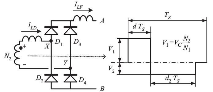
Fig. 7. Voltage shape across winding  $N_2$ .
