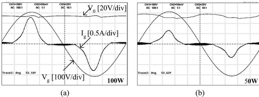
Fig. 19. Input current and output voltage without control loop for the line voltage ( $230 V_{rms}$ ) and  $K = 1$ . (a) Full load. (b) Half load.
