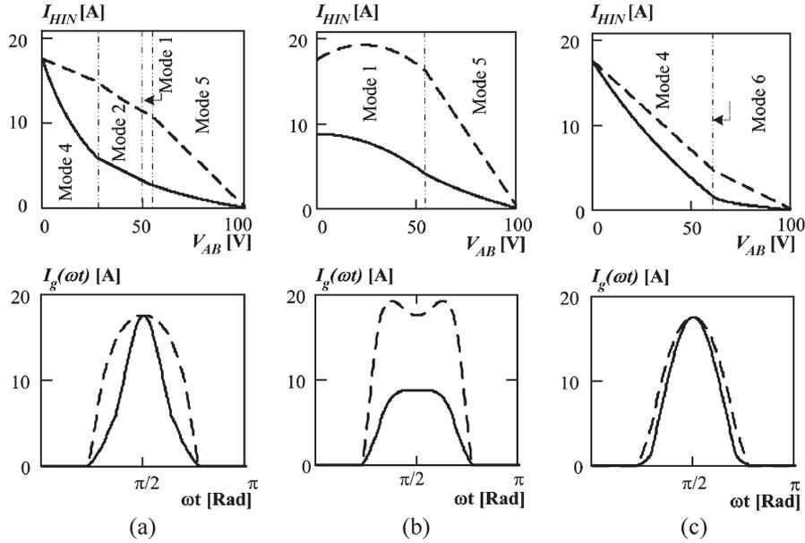
Fig. 13. VCC (peak and average) and input-current shapes (peak and average) for different inductor configurations. (a)  $L_F/L_D = 0.5$ ,  $L_D = 10 \mu\text{H}$ , and  $L_F = 5 \mu\text{H}$ . (b) Only  $L_D$ ,  $L_D = 10 \mu\text{H}$ , and  $L_F = 1 \text{ nH}$ . (c)  $L_F/L_D = 2$ ,  $f_s = 100 \text{ kHz}$ ,  $L_D = 10 \mu\text{H}$ ,  $L_F = 20 \mu\text{H}$ ,  $d = 0.35$ , and  $V_1 = 100$ .
