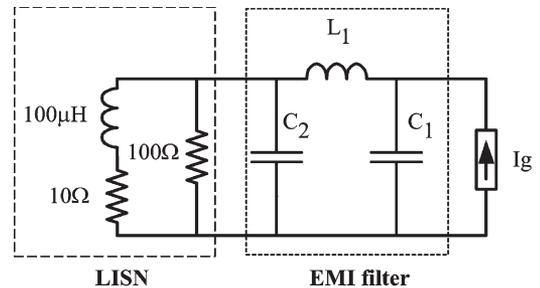
Fig. 15. EMI filter simplified equivalent circuit.
