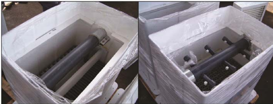
Figure 3: From left to right and up to down: water distribution systems tested; GWSD and PWSD. Schematic arrangement of the water distribution systems tested; GWSD and PWSD.
