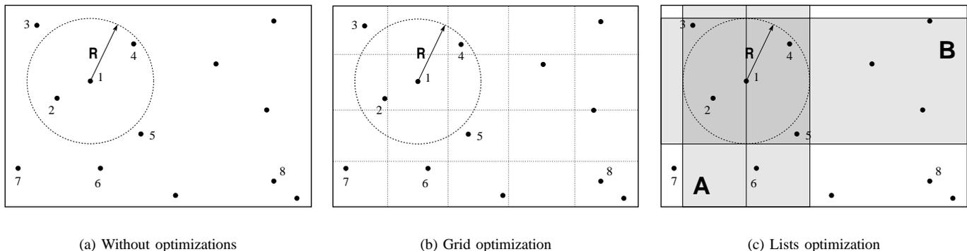
Fig. 3. Propagation computation and optimizations
