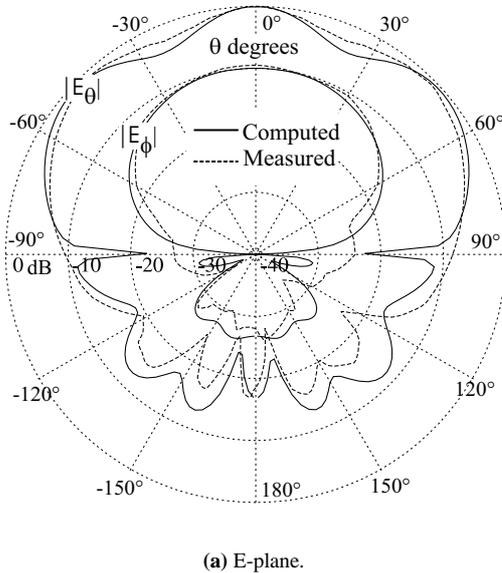
**Figure 12:** Radiation patterns of the printed patch antenna shown in Fig. 4. Ground plane size:  $W_g = 180$  mm,  $L_g = 180$  mm. Frequency is 5.020 GHz. (measurement reproduced from [Bokhari *et al.* 1992])
