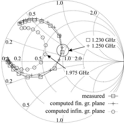
**Figure 9:** Measured versus simulated results for a perfectly balanced patch antenna:  $W_p = W_g = 120.1$  mm,  $L_p = L_g = 79.5$  mm,  $L_p = L_g = 80$  mm,  $X_p = 60$  mm,  $Y_p = 29$  mm. Substrate: RT/DUROID 5870,  $h = 1.57$  mm,  $\epsilon_r = 2.33$ ,  $\tan\delta = 0.0012$ . (increment 2.5 MHz clockwise)
