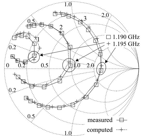
**Figure 8:** Measured versus simulated results for the patch antenna shown in Fig. 4, when the new excitation model is used:  $W_g = 214 \text{ mm}$ ,  $L_g = 214 \text{ mm}$ . (increment 5 MHz clockwise, measurement reproduced from [James and Hall 1989])
