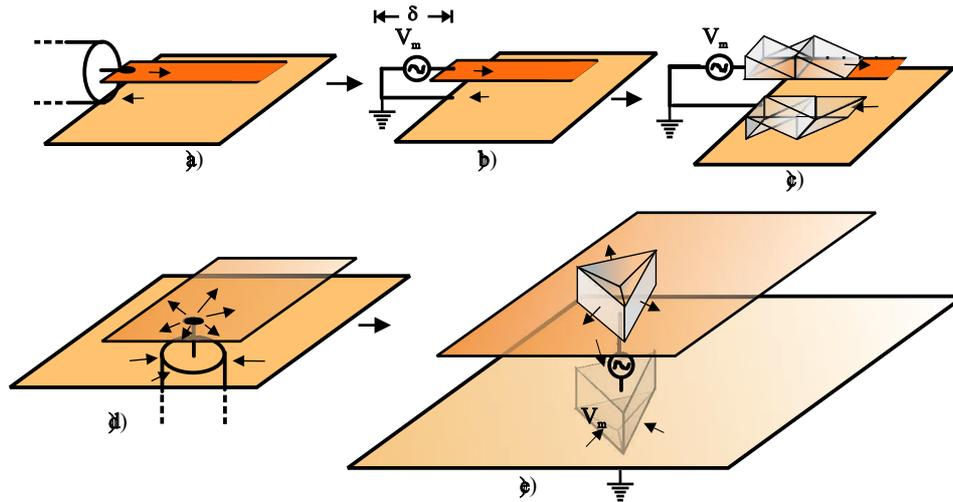
**Figure 7:** Attachment mode for patch antennas on finite ground planes. a) Colinear transition between a coaxial probe and a microstrip line. b) Delta-Gap voltage model applied to a coaxial probe-fed microstrip line. c) Associated MoM description of the excitation model. d) Coaxial probe-fed patch antenna. e) Associated MoM description of the excitation of a probe-fed patch antenna
