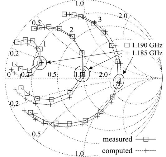
**Figure 5:** Comparison of measured and computed results of the input impedance of the antenna in Fig. 4.  $\square$  measure,  $+$  theory. (increment 5 MHz clockwise, measurement reproduced from [James and Hall 1989])
