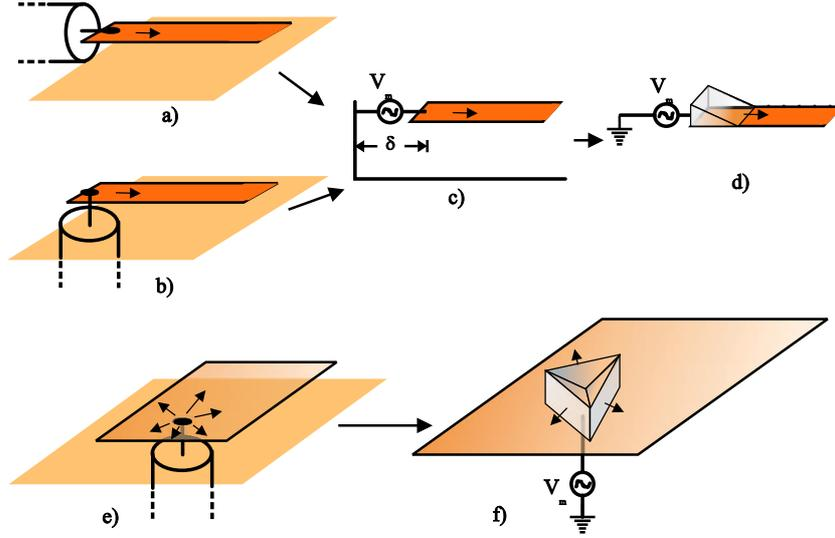
**Figure 2:** A delta-gap voltage source exciting printed circuits. a) Colinear transition between a coaxial probe and a microstrip line. b) perpendicular transition between a coaxial probe and a microstrip line. c) Delta-Gap voltage model applied to a coaxial probe-fed microstrip line. d) Associated MoM description of the excitation model. e) Coaxial probe-fed patch antenna. f) Associated MoM description of the of the excitation of a probe-fed patch antenna
