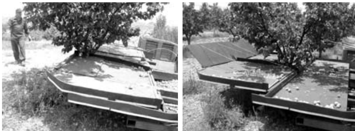
Figure 4. Lower surface extension out (left) and upper surfaces and additional extensions beneath the tree (right).
