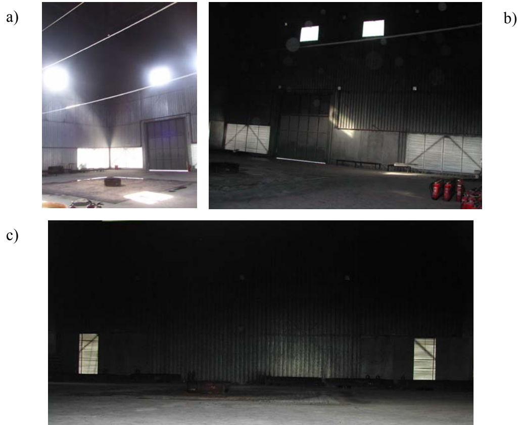
Figure 3. Venting topology of the tests. Test #1: vents open in walls D (D2) and A (A1 and A2), in a), test #2: vents in wall A (A1 and A3 open, A2 closed) in b), and test #3: vents in wall C (C1 and C2 partially open) in c). Views from inside.
