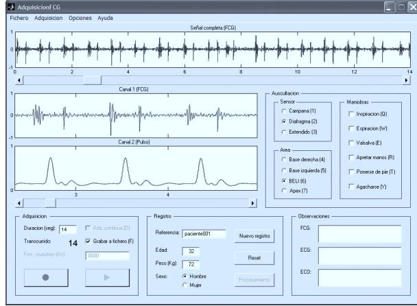
Figure 2. Specific environment for the acquisition of PCG signal.
