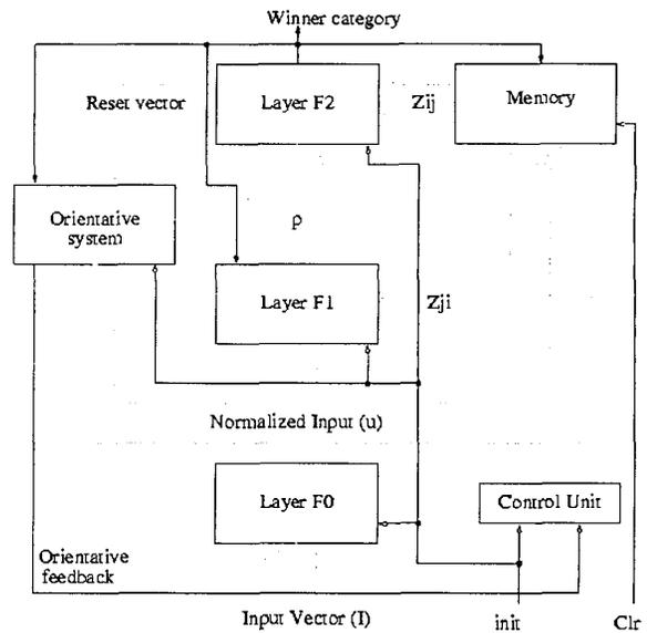
**Figure 1.** Block diagram of the ART2 VHDL-AMS model
