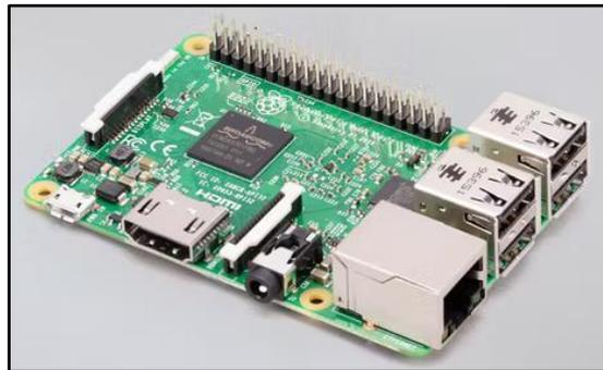
Figura 13. Raspberry Pi 3 Model B
