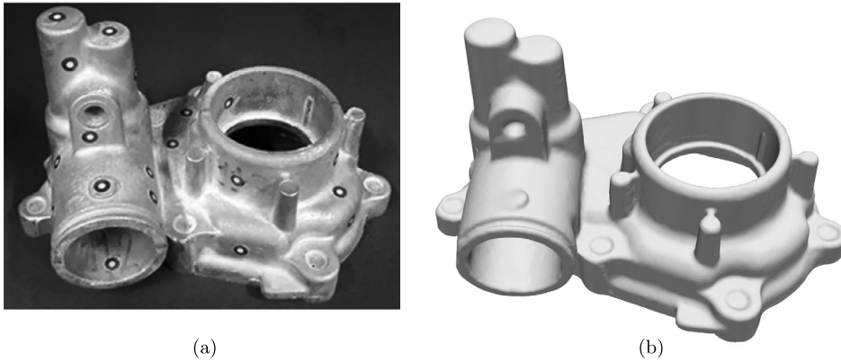
Fig. 21. Aluminum alloy A413 automobile part: (a) real and (b) scanned.
