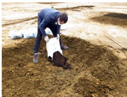
c) Preparation of one of the four paired 2 m x 2 m plots (April 2017) after amendment addition. B: bare soil. AB: amended bare soil.
