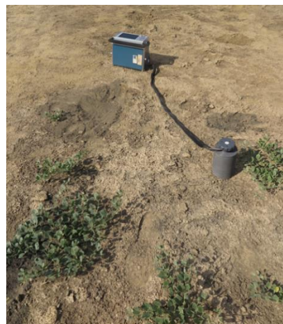
Figure 4.8. Respiration System CIRAS-2 to measure soil CO 2 emission (spring 2018).
