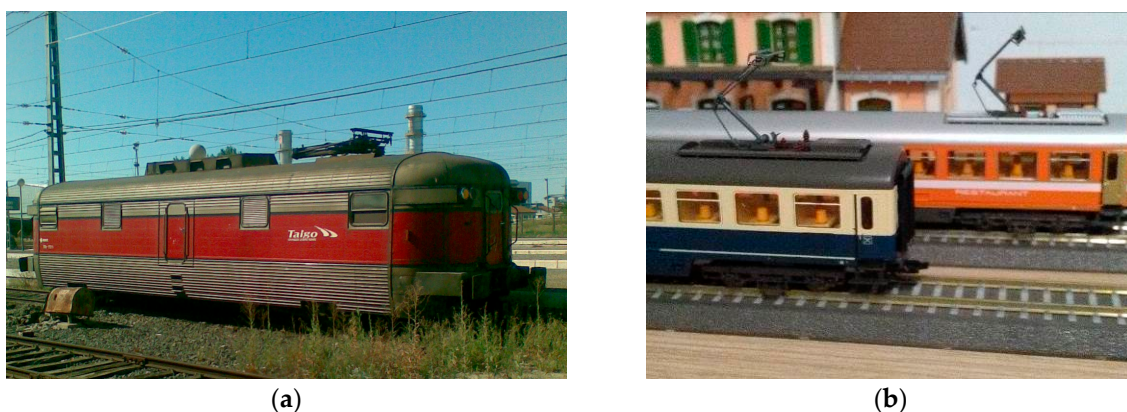
Figure 24. Two examples of the use of pantographs in rolling stock: (a) Former Talgo power-converter coach TG1z for Talgo III series with a “static” pantograph for conversion of 3 kVDC from catenary (static) or locomotive (dynamic) to 380/400 V in case of change of traction or train supply without locomotive; (b) restaurant coaches ARmz of DB (German Operator) and SBB-CFF-FFS (Swiss main operator) with a dynamic pantograph for use in the route.
