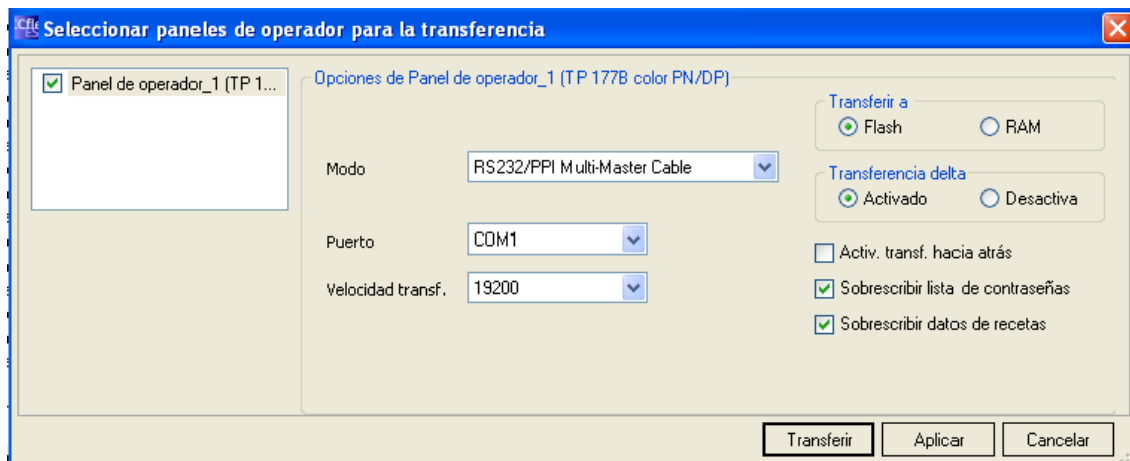
Fig4. 18 Transferencia Software Scada
