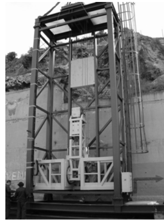
Figure 3. Primary Positioning System with both arm joint (yellow) and joint on tracks (green) of the EFTCoR system
