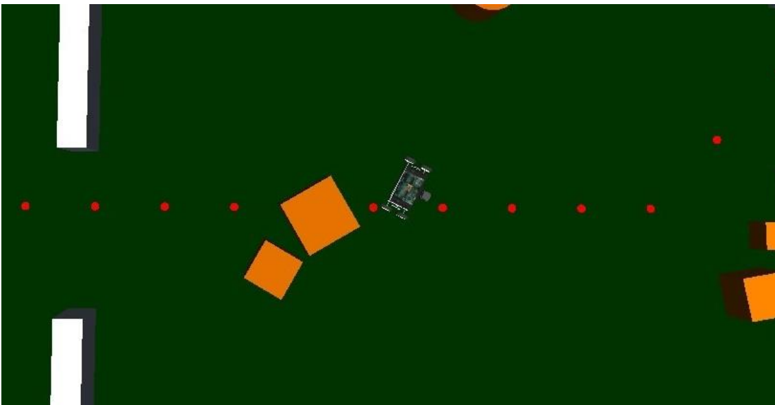
Figure 5.5 Robot re-joins the planned path once past the obstacle
