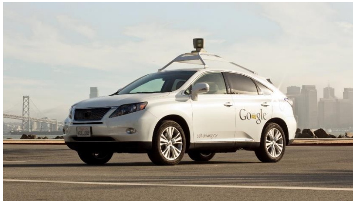
Figure 1.1 Google's self-driving car with LiDAR sensor
