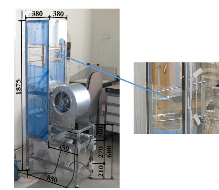
An experimental prototype of a mechanical draft cooling tower has been set up to study the interaction of air and water in a drift eliminators. It consists on a prismatic structure; an airstream is introduced from the bottom of the tower; and a water circuit injects water inside the tower, through one of the plates of the drift eliminator, forming a water film simulating the films formed by the atomization of water in real towers.
