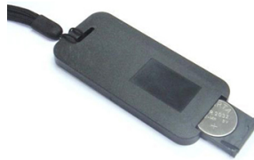
FIGURE 1.2: Example of active transponder with battery supply (Image taken from Veryfields).
