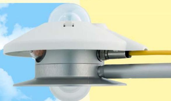
CMA albedometers are suitable for measuring global radiation and/or albedo over many differing types of surface. The upper pyranometer measure incoming global solar radiation and the lower sensor measures solar radiation reflected from the surface below. From the two measurements the Albedo can be simply calculated.
