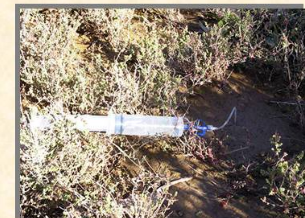
Soil solution was extracted "in situ" using a sampler type Rhizon. Samples were filtered, acidified with three drops of nitric acid and refrigerated until analysis.
