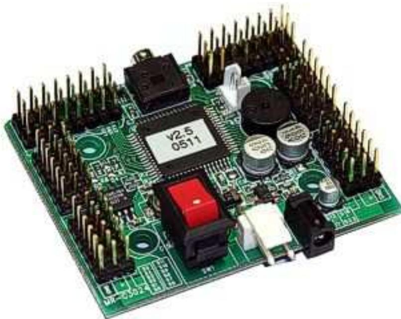
Figura 2.5: Placa base MR-C3024 Robonova-I
