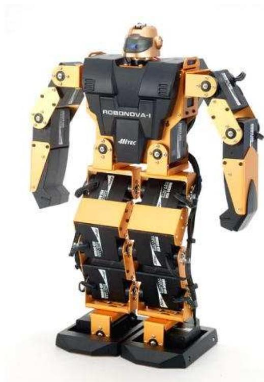
Figura 2.9: Robot Humanoide Robonova-I
