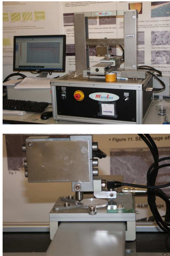
Figura 3.13. Microrayador MTR 3/50-50/Ni de Microtest.
